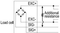
In Case of Adding an Offset Voltage to the Output
